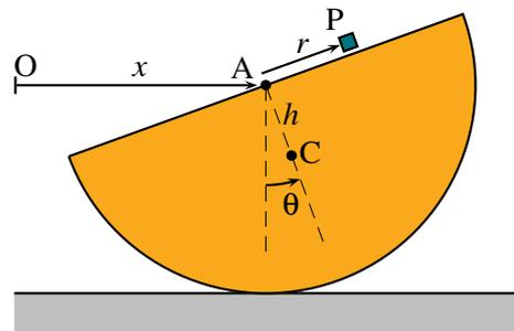
$$\begin{cases} m(\ddot{r} - r\dot{\theta}^2) - ma\ddot{\theta}\cos\theta + mg\sin\theta = 0 \\ [M(a^2 + h^2 - 2ah\cos\theta) + m(a^2 + r^2 + 2mar\sin\theta) + J_C] \ddot{\theta} + [mar\cos\theta + Mah\sin\theta] \dot{\theta}^2 \\ - ma\ddot{r}\cos\theta + 2mr\dot{\theta}(r + a\sin\theta) + Mgh\sin\theta + mgr\cos\theta = 0 \end{cases}$$
